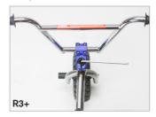
Once any 'rock' has been dialled out from the headset, check your bars turn freely left to right, then tighten your stem pinch bolts nice and tight.
