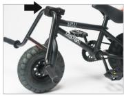
With the left pedal installed you can now stand the bike up using the pedal as a bike stand. This makes the job a lot easier. Now install the right hand pedal (marked 'R'), this time the pedal is turned clockwise to tighten. Again be careful not to cross thread the pedal and make sure the pedal is done up nice and tight.
