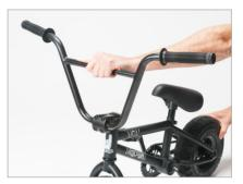
If there is excessive play, you can remove it by lightly tightening your headset pre load bolt (stem pinch bolts MUST be loose during this operation then re-tightened to check for headset play).
